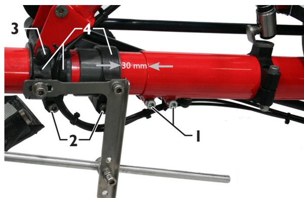
6. Using a 6mm Allen key, tighten the bolt (3) on the front clamp lightly, ensuring that the steering/crank column can still be easily tilted to the side. Tighten the bolts (2) on the rear clamp (using a 6mm Allen key) then loosen them for 1/8th-turn and lock them with the headless screws coming from the side.
