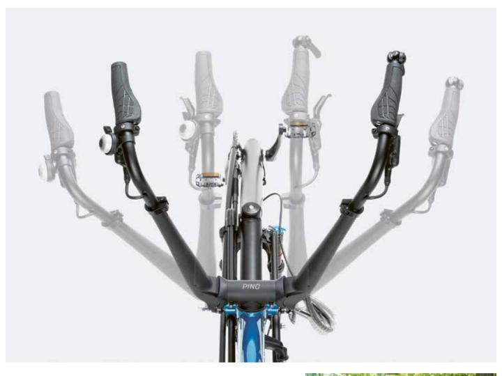
The picture that looks like a huge set of mechanical antlers is actually a photomontage of the PINO's new handlebars shown in various positions. For improved ergonomics, the handlebar width can be adjusted – without having to change the grip angle. The new handlebars are even height-adjustable. With this ingenious design, riders of any size and stature will be able to find the perfect handlebar position.
