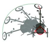
> Thanks to its geometry, a delta trike can turn on a dime – which can also be helpful when parking.
