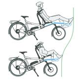
> The PINO can be infinitely adjusted to accommodate riders as tall as 6'7" (2 m) in height or – with the length-adjustable crank arms and an adapter – as small as 3'3" (1 m).
