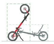
> Upright parking allowed! A delta trike can be parked with its front wheel in the air, which saves space indoors and is a real eye-catcher outdoors.
