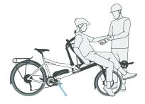
> The PINO rests safely and securely on its double kickstand, even when loaded. This makes it easy for the rear rider to help a front passenger get into and out of the seat.
