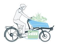
> The foldable Porter Bag transforms the recumbent seat into a shopping bag with a capacity of 120 liters. The Porter Rack can hold bulky and heavy cargo items – e.g. two beverage crates.
